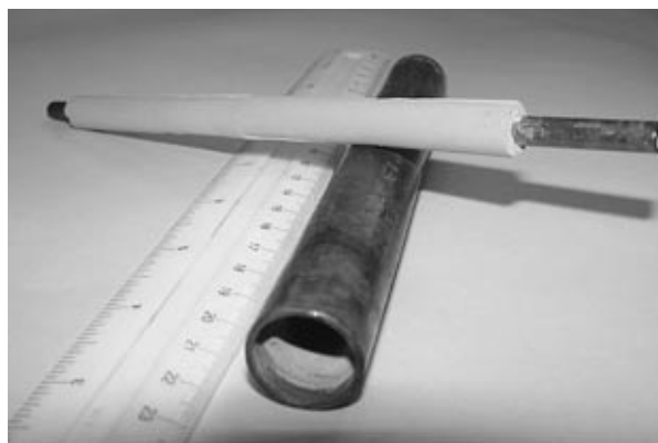
Fig. 17. Samples of composite coatings on the inner and outer surfaces of metal tubes.
